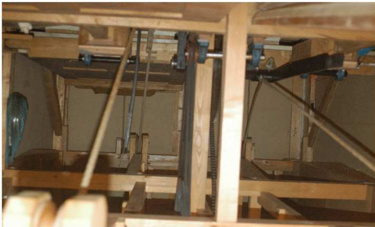
Automatic pull-bellows (mode “a”) , simulating the human manual action
